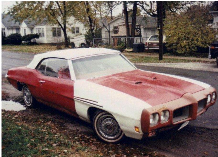
We drove the car in this configuration for a couple of years, and learned that the manual drum brakes were not too good, the 4-speed shifted poorly, and the motor was so loose that when we'd rev it up past about 2,500 RPM the timing chain would sling out so wide it would rub against the insides of the timing cover! The motor was so loose that I hardly ever left the city limits with it, but we had a running GTO Convertible!
